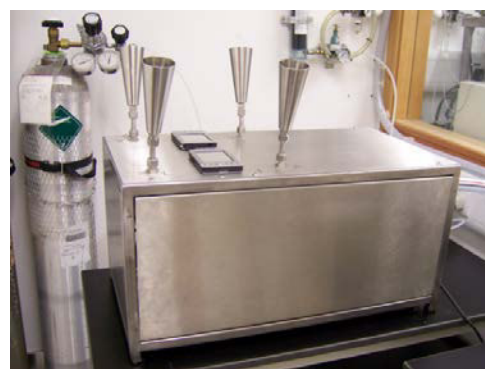
Olfactometer in PolyU (Olfactomat-n2)
