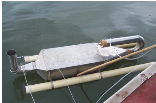
Wind tunnel for odour sampling
