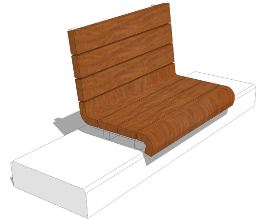
Fig. A-33 Seat on concrete bench
